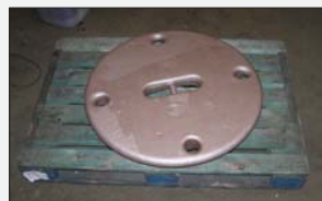
Fig. 6. The system is designed for transport on euro pallets for easy transport to new locations or to service. Part of the bottom weight is shown.
