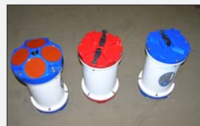
Fig. 7. Current speed and direction as well as wave height and direction is measured using a sea floor mounted ADCP (left). ADCP = Acoustic Doppler Current Profiler. An under water data processor (right) delivers processed data in near real time. The unit in the middle contains batteries.
