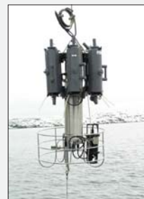
Left: CTD with sampling bottles, and in situ chlorophyll fluorometer. Top right: A helicopter is used for water sampling in Schleswig-Holstein. Right: Tube sampling is often used in Sweden.
