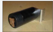
Fig. 4. A combined sensor for chlorophyll a and turbidity. The optical window is covered with a copper shutter when the instrument is idle.
