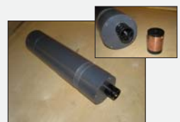
Fig. 5. Nitrate is measured using a method without chemicals. The absorption in UV-light is used for quantification. A copper cage is used to reduce bio-fouling problems. Detection limit is higher and accuracy lower compared to wet chemical techniques.
