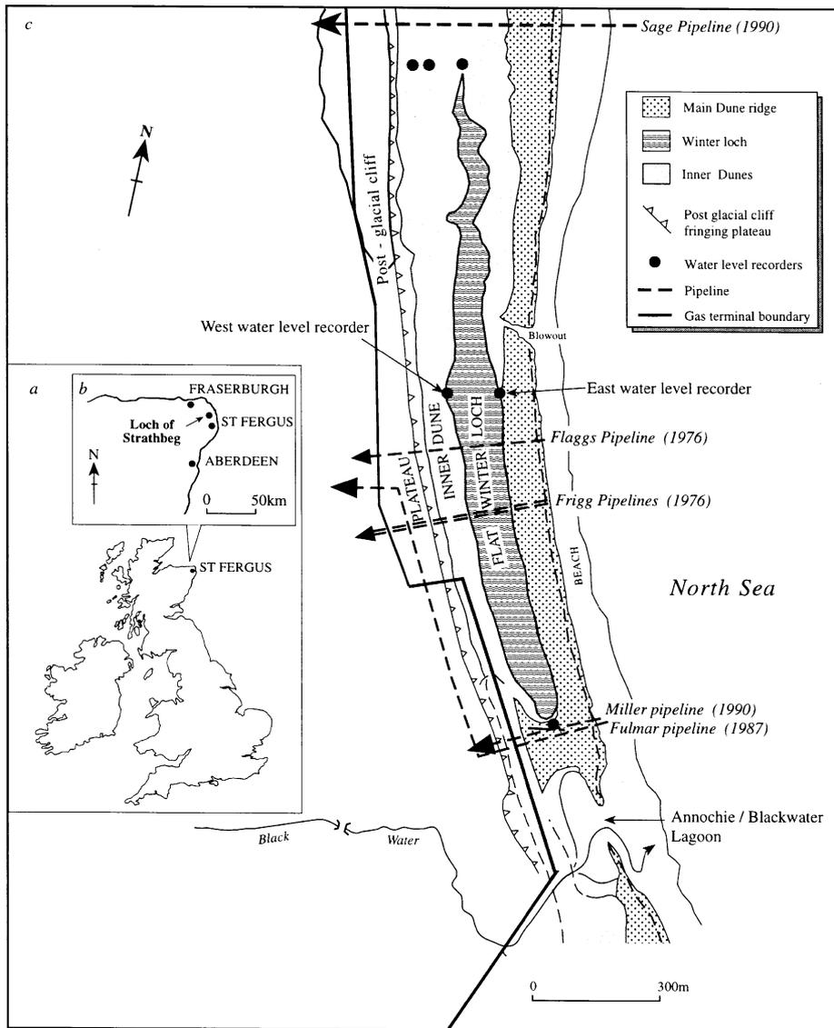
**Fig. 1.** a. Location of the study area; b. St. Fergus site; c. main features, instrumentation and pipeline location (with year of construction) at the St. Fergus dune system. d. Air photograph of the St. Fergus dunes with gas terminal behind the dunes.
